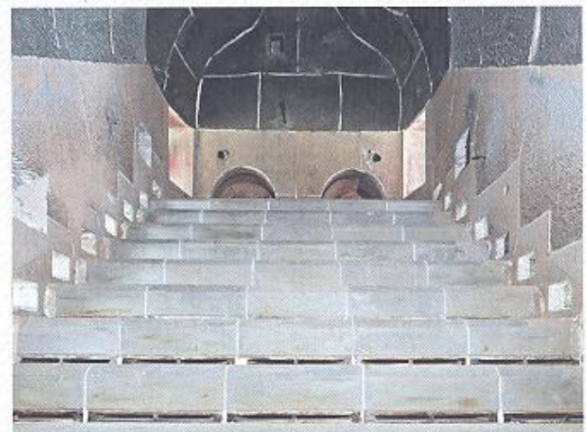
// Page 64 PREPOL Step Combustor (SC) – a simple combustion system for solid alternative fuels
